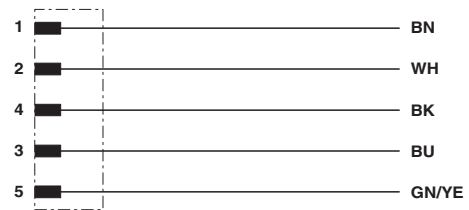
Contact assignment of the M12 plug
