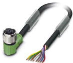
Sensor/actuator cable, 8-position, Variable cable type, free cable end, on Socket angled M12 SPEEDCON, A-coded, cable length: Free input (0.2 ... 40.0 m)
