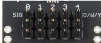
The Motion Board supports up to 5 servo motors. The servo motors can be either standard motion or continuous rotation servos. There's a note on the board ("O/W/Y") for the color which should be on the top row of the header: orange, white, or yellow. Most servo motors will have one wire which is one of these colors, and that wire should line up with this note.
