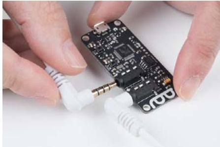
Plug the end of this cable into the audio output jack on your phone, tablet, or whatever device you're using to program the system.
