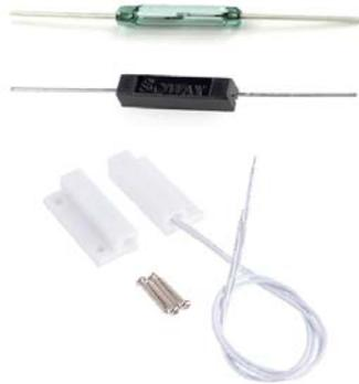
*From top to bottom: A glass PTH reed switch, an insulated plastic PTH reed switch, and a reed switch designed for doors and windows. If you look closely at the center of the top, glass switch, you can see the metal arms inside.*
